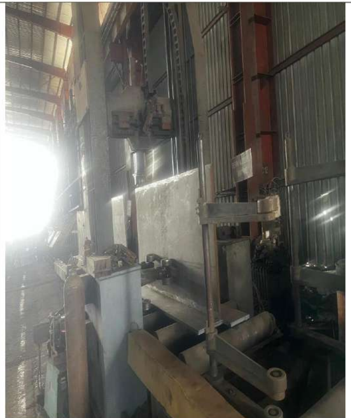
BEAM FITUP MACHINE
